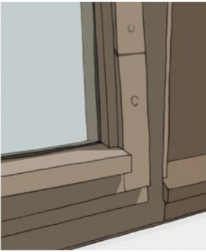
② Small Sections Where there are short sections of degraded timber, a new section of timber will be spliced in.
